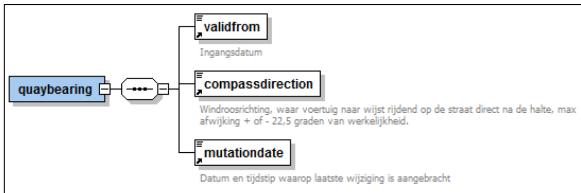
Figuur 13 XSD Quay-bearing
